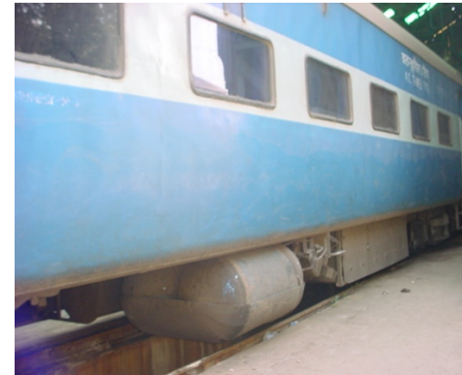
Under Slung Water Tank
